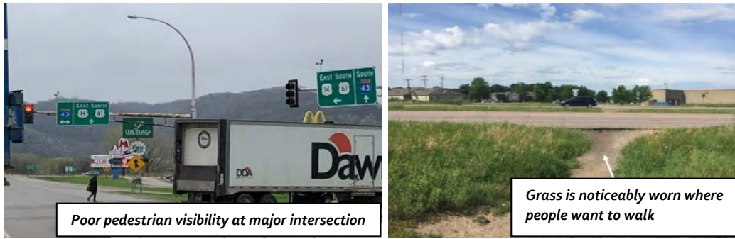
Figure 6. Factors to consider when conducting a scoping walk. Left: Limited visibility. Right: Uncontrolled crossing location. Photo source: MnDOT
